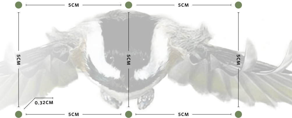
[FIG 1] Diagram of bird friendly glazing pattern with visual markers at maximum 5cm x 5cm spacing IMAGE SOURCE: FLAP CANADA
