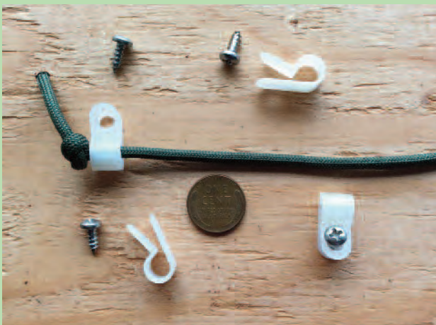
1/4” Cable Clamps supporting custom-made BirdSavers
